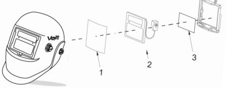
1) Outer screen guard : if this screen is dirty, damaged or scratched, Bollé Safety recommends you change it. Ideally, the screen needs to be changed weekly (1 time / week) (ref. COVFUSPEXT).
