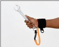
Always check the hook-and-loop closures fasten properly, as they guarantee that the bracelet stays closed and holds if the tool is dropped.
