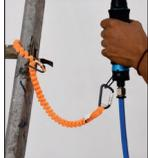
Always check the connectors are closed and locked.
